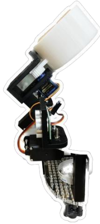
Figure 89: Gripper Arm Structure with Support Mechanism
