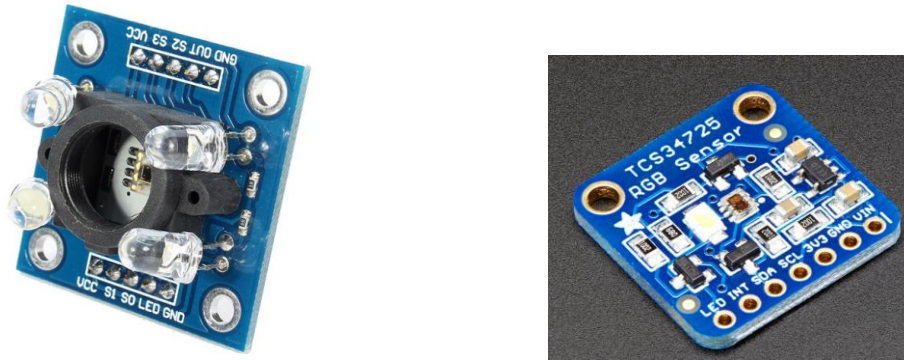
Figure 64: Comparison of TCS3200 Color Sensor and TCS34725 Color Sensor [28]
